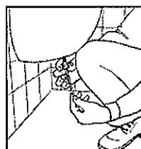
**10- Install the clamping nut to the screw and fix it manually.**
