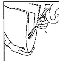
**8- Pass the screw tap through the hole beneath the half-pedestal.**
