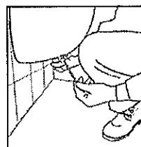
**11- By holding the nut, the screw tap is demounted from its cap in the screw. (Keep the screw tap, you may need it again!)**
