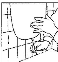
**9- Install the half-pedestal against the basin and draw the screw tap downwards.**
