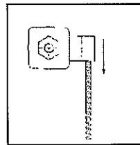
**4- When the fixing process is over, the direction of the nut should be downwards, not indicating left or right.**
