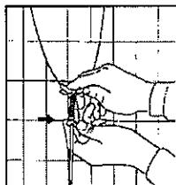
**6- The clamping nut is demounted.**
