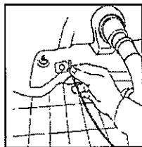
**3- Settle the metal plate to prevent the sliding of the appliance during the fixing process. Insert the nut and fix it with a wrench.**
